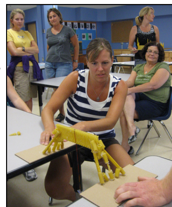
Strength of a pasta bridge is tested using a bucket of sand during an engineering challenge at training provided by The WORKS.
